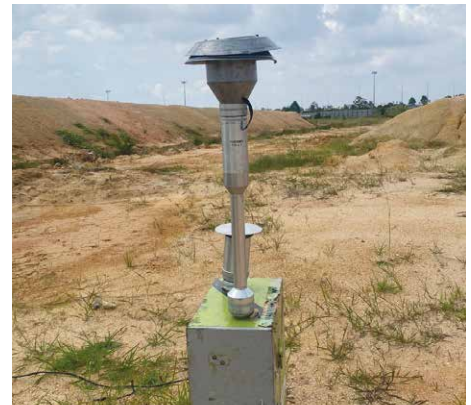
High-volume air sampler used to monitor particulate matter at our construction sites
