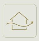
Hot air naturally rises, hence we have designed your home to draw in natural air while allowing hot air to escape via cross ventilation from the windows. By carefully placing window openings towards the direction of prevailing winds, natural cooling air can be ventilated throughout the home.
